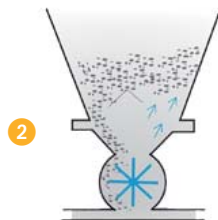
The material is directly blown into the blow-through rotary valve
