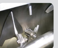
Liquid injection device
