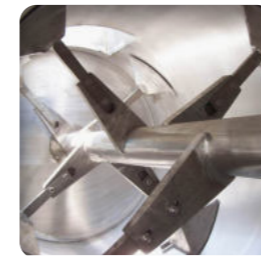
▶ Low maintenance: easy cleaning and access to all the internal parts of the mixer
