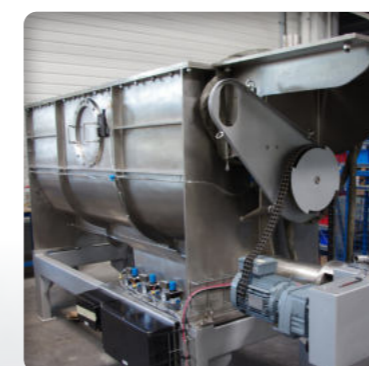
▶ Chain drive of the agitation device
