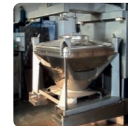
Secured locking of the container for mixing without any risk to operators
