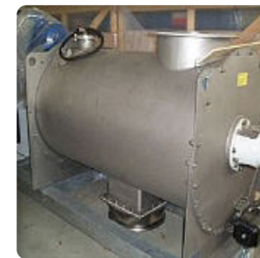
▶ Stainless steel cylindrical mixer
