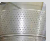
Double casing heating/cooling
