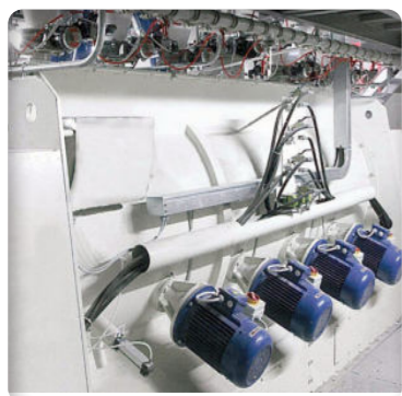
▶ Multi-choppers mixer for incorporation of high proportion of liquid
