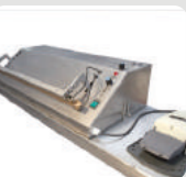
Welder for inner liner
